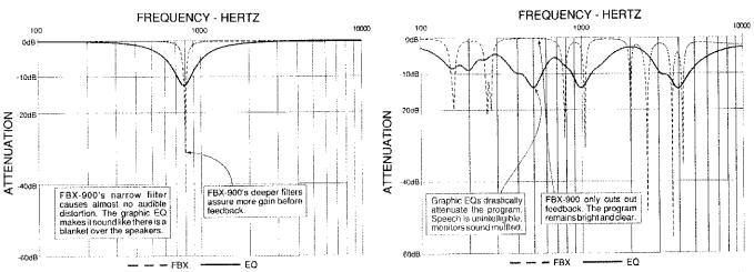
Full Set-Up Test Procedure: A PA system was set up using a microphone, mixer, FBX-900, power amp, and two speakers. The system's gain was raised until the FBX-900 removed nine feedback points. Next, the FBX-900 was replaced with a 1/3 octave graphic EQ. The EQ was adjusted while the system gain was raised to the same level achieved with the FBX. The frequency response curves of each device was then plotted.
